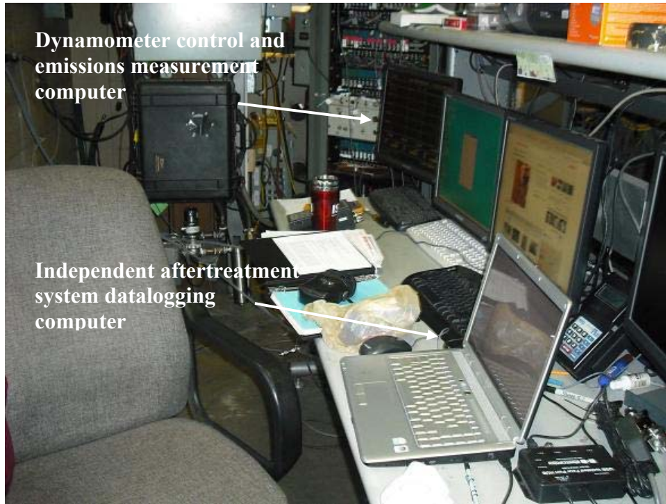
Figure 24. WVU EERL control console area
