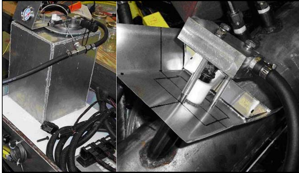
Figure 12. Urea-SCR system urea dosing hardware
