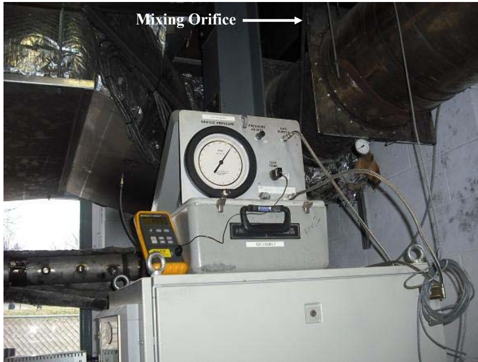
Figure 20. Propane injection kit connected to dilution tunnel
